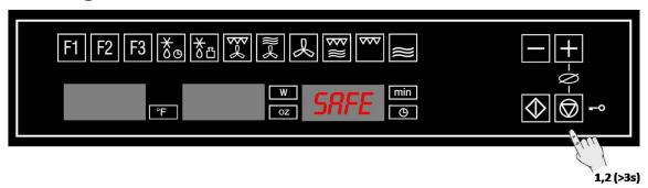
The oven functioning can be blocked (for example, to stop it being used by children).
